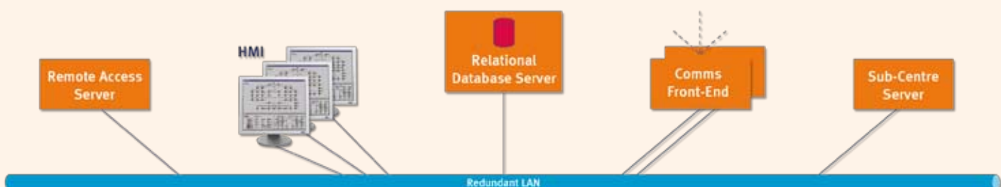
Typical Control Centre Architecture
